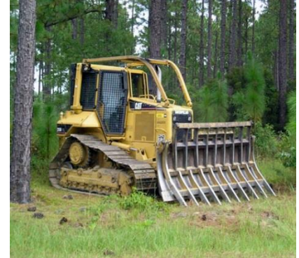
Figure 6. Bulldozer with Brush Rake (Photo Credit FPC)
