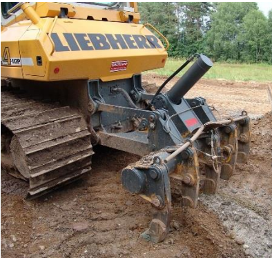
Figure 4. Bulldozer with Root Ripper (Photo Credit FPC)
